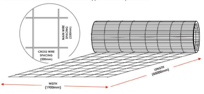
Plain welded steel fabric bonds to concrete by the positive mechanical anchorage at each intersection. Roll welded steel fabric achieves bonding and anchorage with welded intersections.
