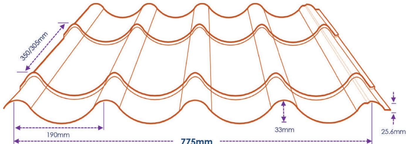
**TOLERANCES:** Length: 0-10mm | Width: +/-3mm | Thickness: +/-0.03mm
