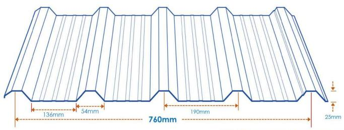
TOLERANCES: Length: 0-10mm | Width: +/-3mm | Thickness: +/-0.03mm
